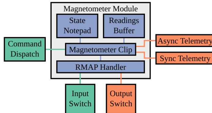
Figure 6-12: Magnetometer Module Structure
