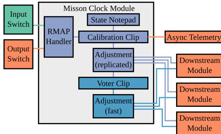
Figure 6-15: Mission Clock Module Structure
