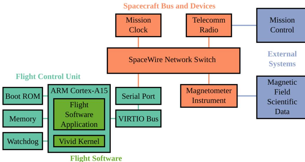
Figure 5-1: Testbench Spacecraft Avionics
