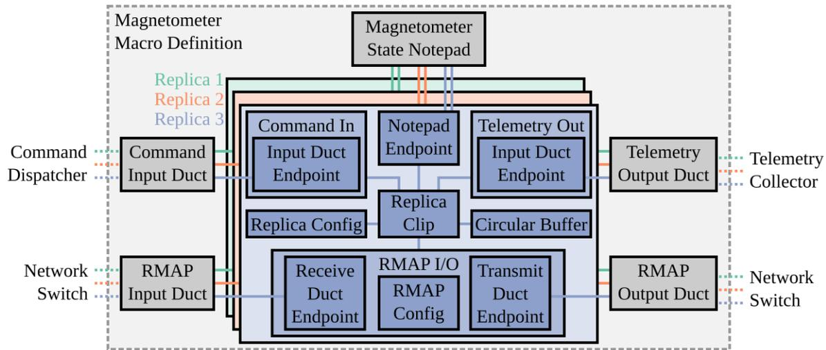
Figure 3-6: Example Replicated Magnetometer Component
