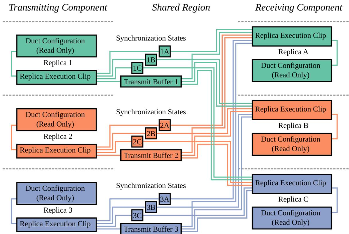
Figure 3-5: Example 3x3 Voting Duct Connectivity Diagram
