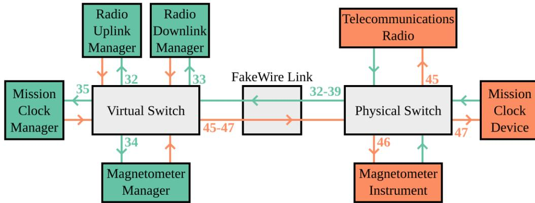
Figure 6-6: Complete SpaceWire Network Map
