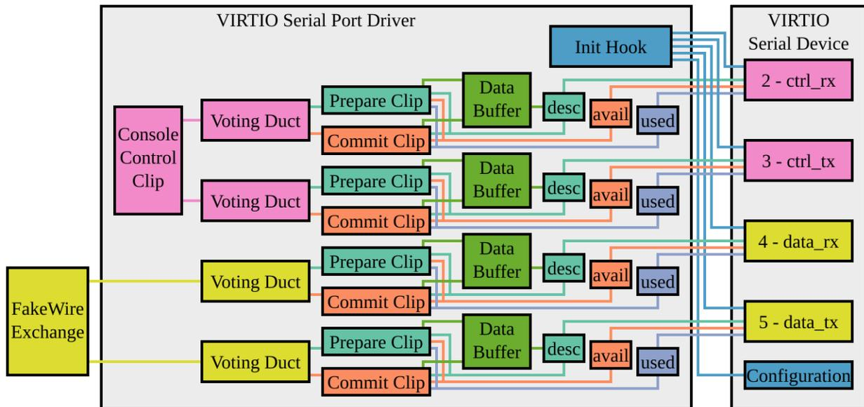
Figure 6-2: VIRTIO Driver Structure
