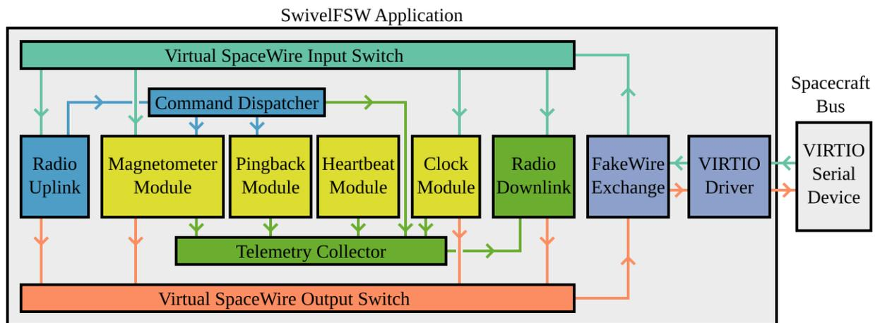
Figure 6-1: Overview for the SwivelFSW Flight Software
