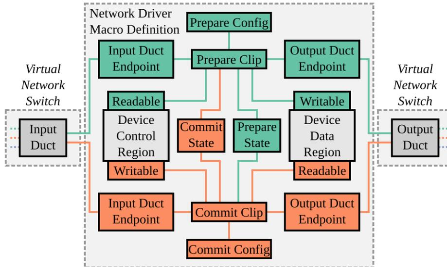
Figure 3-7: Sample Network Device Driver using Prepare/Commit Replication
