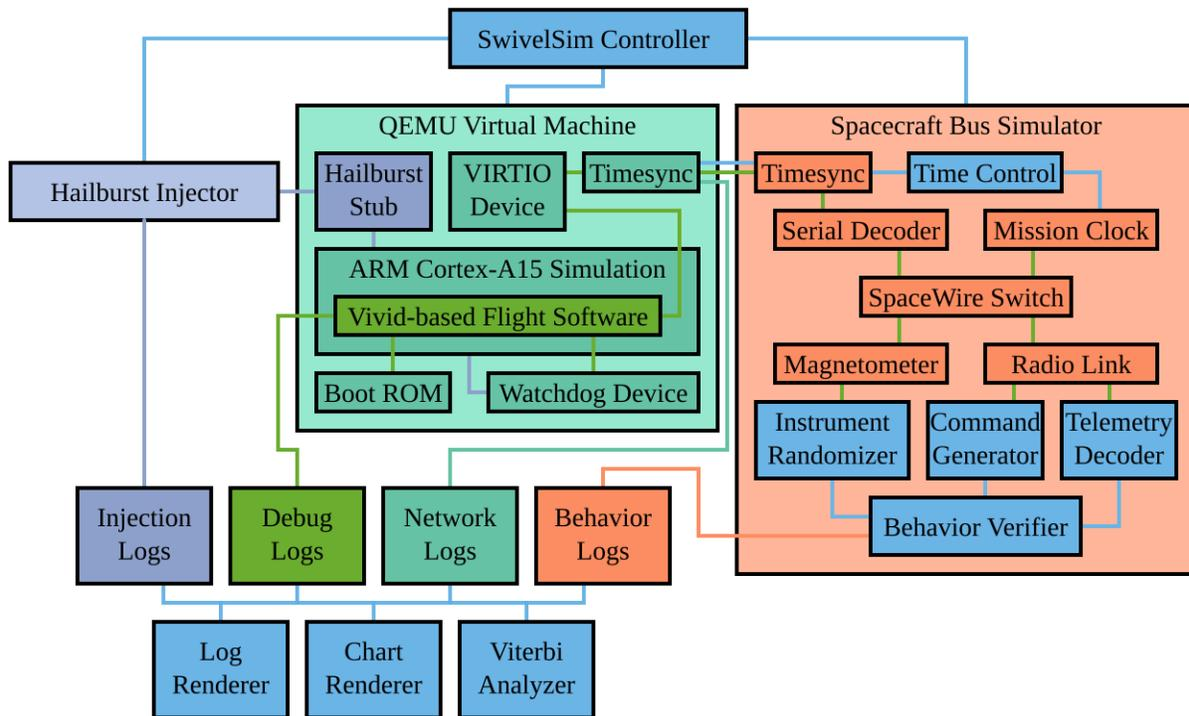
Figure 7-1: SwivelSim Simulation Overview
