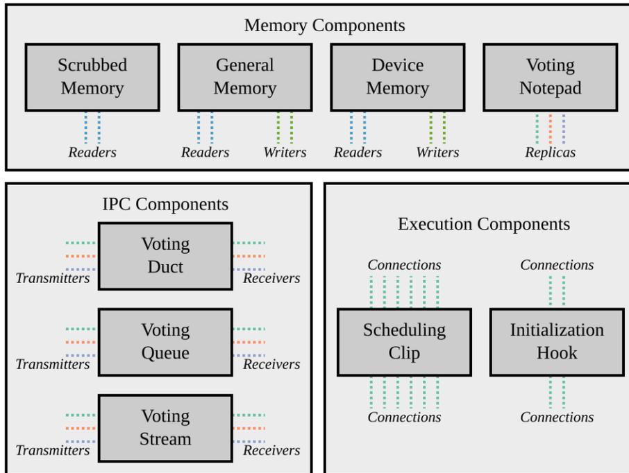
Figure 3-3: An overview of Vivid's core components
