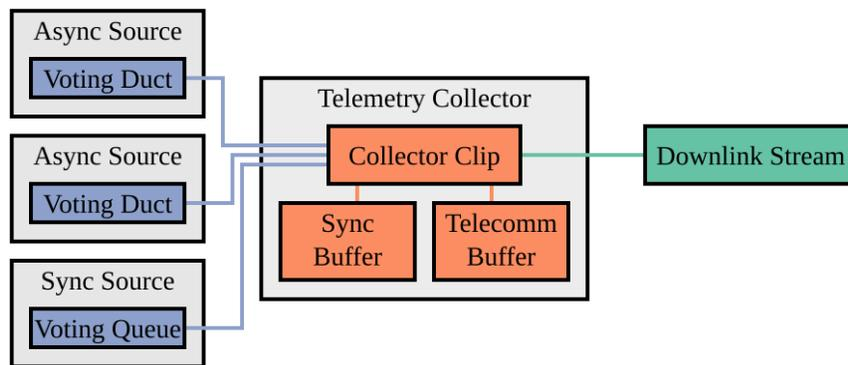
Figure 6-11: Telemetry Collector Structure
