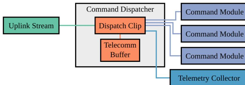
Figure 6-10: Command Dispatcher Structure
